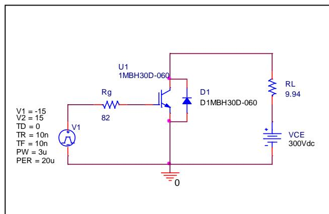
Test condition: IC=30 (A), VCC=300 (V)
