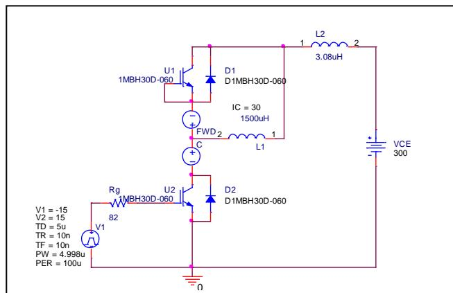
Test condition: Vcc=300 (V), IC=30 (A)  $-di/dt=90$  A/usec
