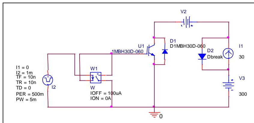
Test condition:  $V_{CC}=300$  (V),  $I_C=30$  (A),  $V_{GE}=15$  (V)
